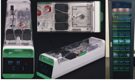
(a) The CL1 biocomputer platform includes an integrated microelectrode array(MEA) and perfusion system for maintaining neuronal cultures. Adapted from [13].
