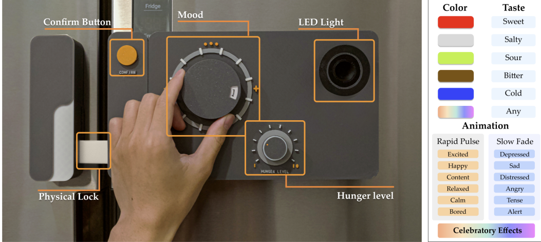
Figure 3: Left: physical interface components. Top right: light colors evoke taste via synesthetic associations. Bottom right: light animations reflect mood and celebrate progress.
