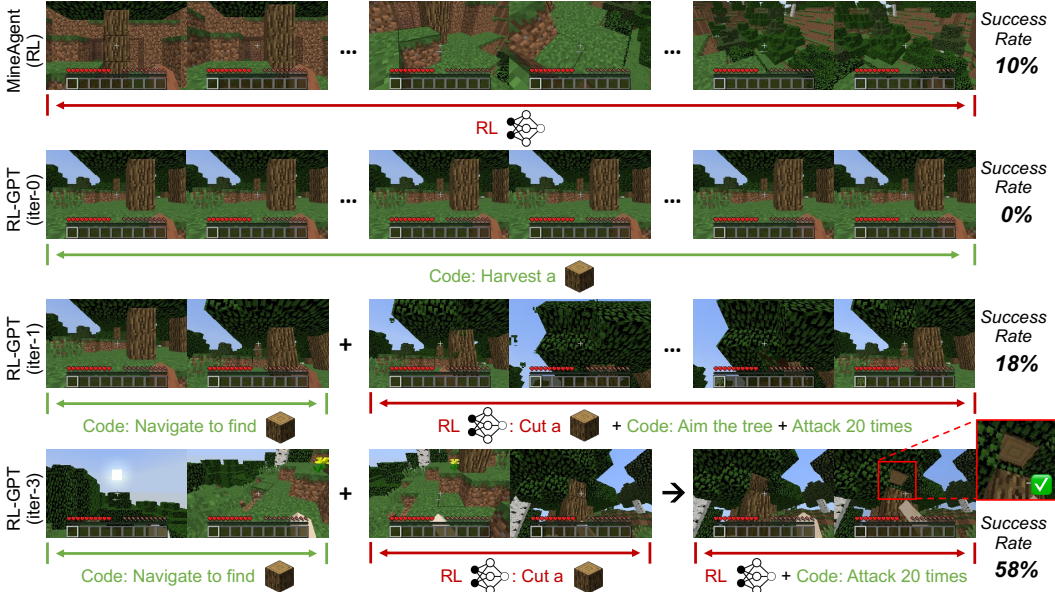
Figure 5: Demonstrations of how different agents learn to harvest a log. While both RL agent and LLM agent learn a single type of solution (RL or code-as-policy), our RL-GPT can reasonably decompose the task and correct how to learn each sub-action through the slow iteration process. RL-GPT decomposes the task into “find a tree” and “cut a log”, solving the former with code generation and the latter with RL. After a few iterations, it learns to provide RL with a necessary high-level action (attack 20 times) and completes the task with a high success rate. Best viewed by zooming in.
