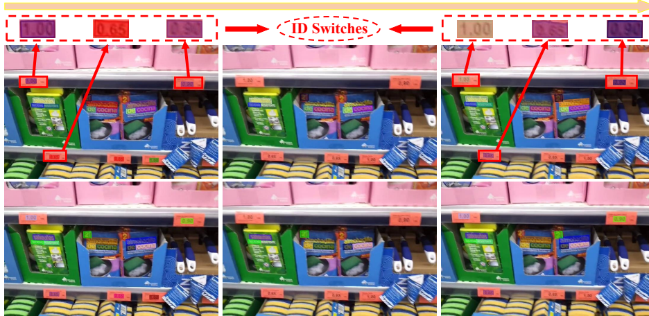
Figure 5: Visualization results of ST-Matcher and LST-Matcher. The first row shows the failure case that suffers from the ID switches issue when using only ST-Matcher, caused by missed detection and erroneous matching. The second row shows that LST-Matcher effectively mitigates this issue via both long and short term matching. Text instances in the same color represent the same IDs.
