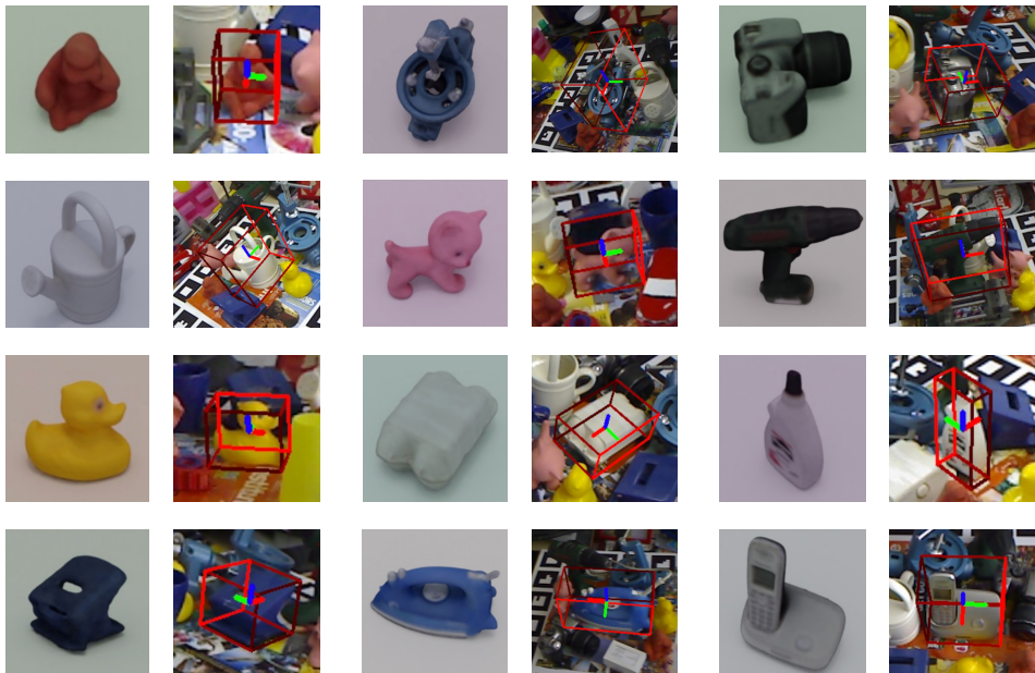
Figure 14: Qualitative results of VFM-6D on LINEMOD. For each object instance, the left image is the reference image found by VFM-6D. The right image is the corresponding query image, on which the object pose estimation results are overlaid.
