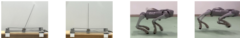
Figure 3: Left : Cartpole task in reality, aiming to keep the pendulum on the cart balanced for as long as possible. Right : Go2 task in reality, aiming to keep running forward and track a specified speed.
