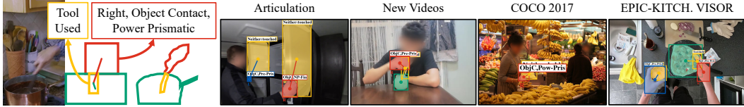
Figure 1: (Left) The rich output of our model, consisting of boxes and segments for hands ( left hand blue , right hand red ), objects in contact , as well as second objects that are contacted by a tool. Output includes contact, making distinctions between touching and holding as well as grasp type. (Right) The method is powered by new annotations on new and existing data, covering many scenarios. Results shown are selected outputs on our test set.
