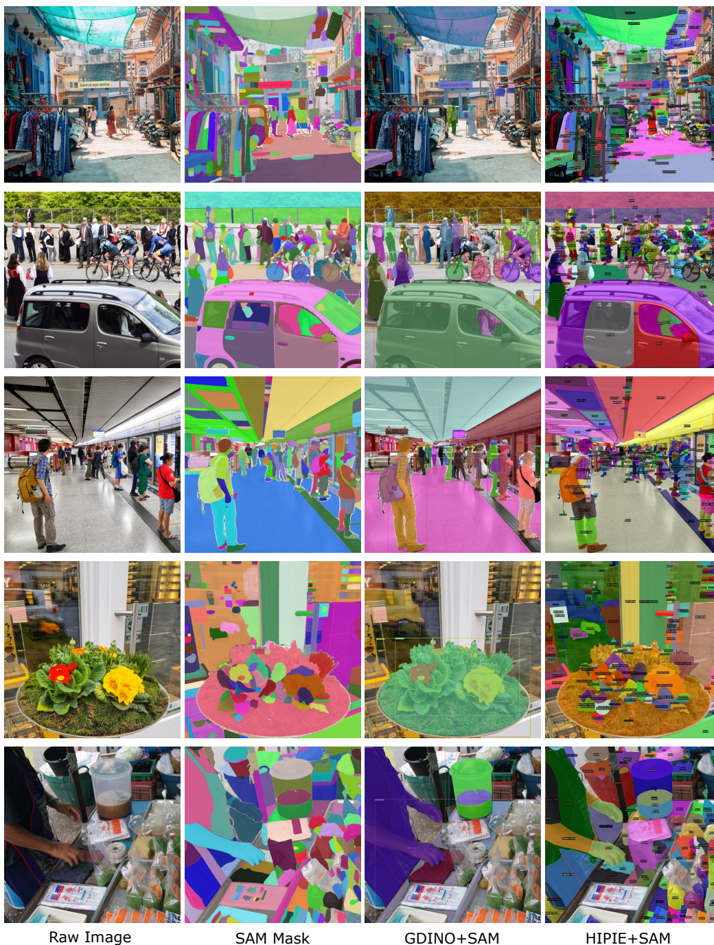
Figure A6: Additional results of merging HIPIE with SAM for hierarchical segmentation. By integrating the part masks from our model and conducting a vote among SAM’s panoptic masks, we generate finely detailed mask outputs. Our method demonstrates fewer misclassifications and overlooked masks across the SA-1B dataset compared to the Grounding DINO + SAM approach. Furthermore, our technique excels in differentiating between intra-class objects and identifying distinct object parts.
