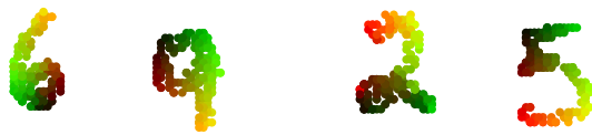
Figure 6: Left image: Matching of the numeral "6" to the numeral "9". Right image: Matching of the numeral "2" to the numeral "5". The colors represent which point in one numeral corresponds to another point in the other numeral.
