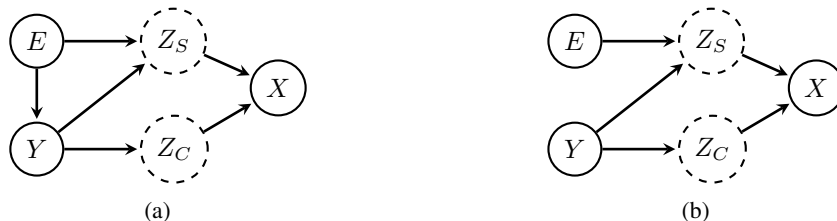
Figure 2: a) Causal Directed Acyclic Graph (DAG) we consider in this work. Solid nodes are observed and dashed nodes are unobserved. We assume an anti-causal setting where label Y causes X , and X has 2 causal parents: “style” features, Z_S , which are influenced by the environment E ; and environment-independent “content” features of X , Z_C , which are causally influenced by the label Y . E potentially influences Y . Both E and Y have direct influence on style features Z_S . b) Same DAG as a) with an intervention on Y . We note that Y \perp\!\!\!\perp E \mid Z_C and Y \not\perp\!\!\!\perp E \mid Z_S .
