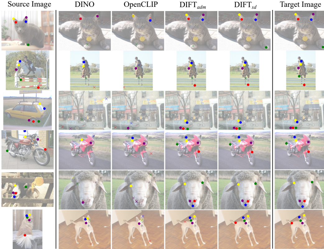
Figure 3: Visualization of semantic correspondence prediction on SPair-71k using different features. The leftmost image is the source image with a set of keypoints; the rightmost image contains the ground-truth correspondence for a target image whereas any images in between contain keypoints found using feature matching with various features. Different colors indicate different keypoints. We use circles to indicate correctly-predicted points under the threshold \alpha_{bbox} = 0.1 and crosses for incorrect matches. DIFT is able to establish correct correspondences under clustered scenes (row 3), viewpoint changes (row 2 and 4), and occlusions (row 5). See Fig. 17 in Appendix E for more results.
