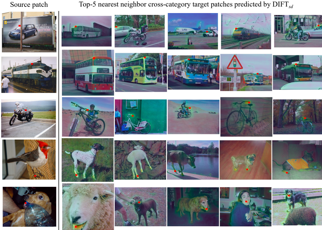
Figure 18: Given the image patch specified in the leftmost image (red dot), we use DIFT_{sd} to query the top-5 nearest image patches from different categories in the SPair-71k test set. DIFT is still able to find correct correspondence for object parts with different overall appearance but sharing the same semantic meaning, e.g., the leg of a bird vs. the leg of a dog.
