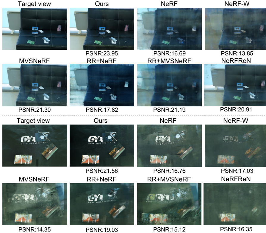
Figure 4: From left to right: the target view, our results, the results obtained by NeRF [1], NeRF-W [7], MVSNeRF [10], RR+NeRF [1], RR+MVSNeRF [10], and NeRFReN [32]. The target views in the two scenarios (scenes with detachable glass, captured with the similar setup as [6]) are obtained by removing the glass, and are compared with the results as ground truth for PSNR values shown below each image. Please zoom in for more details.
