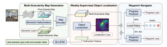
Figure 2: General scheme of WS-MGMap for VLN task. We assemble both fine-grained details and semantic information about environments to build a multi-granularity map. Agents learn to leverage such information for representing diverse objects through a weakly-supervised object localization task. The learned map and instruction are then fed to a waypoint navigator for deciding actions.
