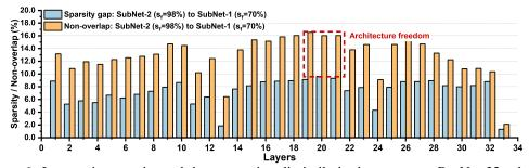
Figure 6: Layer-wise sparsity and the connection dissimilarity between two ResNet-32 sub-nets trained by the non-disjoint (ND) AST scheme.
