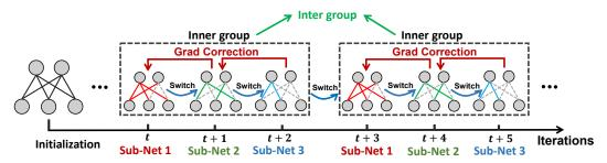
Figure 3: The overview of the AST process with gradient correction on consecutive inner-group sub-nets (AST-GC)
