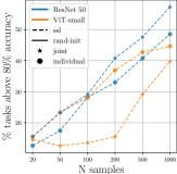
Figure 6: **Sample efficiency**: The percentage of tasks for which performance is above 80% plotted against the number of training samples per task rule, with random initialization (top) and with SSL pre-training (bottom).
