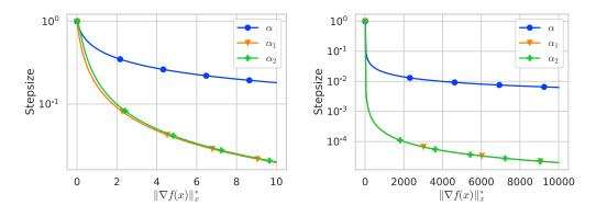
Figure 3: Comparison of stepsizes of affine-invariant damped Newton methods with quadratic local convergence. We compare AICN (blue), and stepsizes from Nesterov [2018] in orange and green. We set  $L_{\text{semi}} = L_{\text{sc}} = 5$ .
