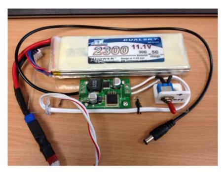
Figure A2.4: The lithium power source. Since ODROID XU3 is running on 5 volts, a voltage regulator (the green board) is added to convert the 11.1 volts from the lithium battery. Battery specifications: 11.1V, 2300 mAh, 30 C, Li-Polymer battery.
