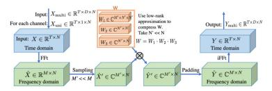
Figure 5: Structure of Frequency Enhanced Layer (FEL): Original version (use weights W) and Low-rank Approximation version (use weights  $W = W_1 \cdot W_2 \cdot W_3$ ), where N is Legendre Polynomials number, M is Fourier mode number, and T is sequence length.
