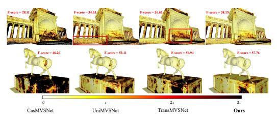
Figure 6: Comparison of reconstructed results with our baseline [7] and top-2 published models [19, 3] on Tanks and Temples benchmark [9]. The first row shows Recall on the advanced scene of Temple ( $\tau = 15mm$ ); the second row shows Recall on the intermediate scene of Horse ( $\tau = 3mm$ ).
