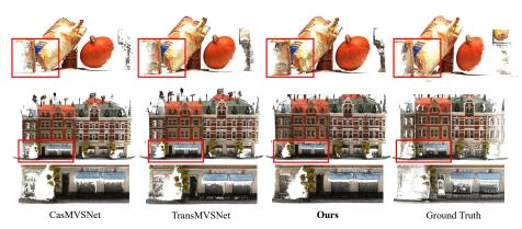
Figure 5: Visualization comparison with state-of-the-art methods on DTU evaluation dataset [8] (scan15 and scan32). Compared with our baseline [7] and TransMVSNet [3], our WT-MVSNet obtains a more complete point cloud shown in the red bounding boxes.
