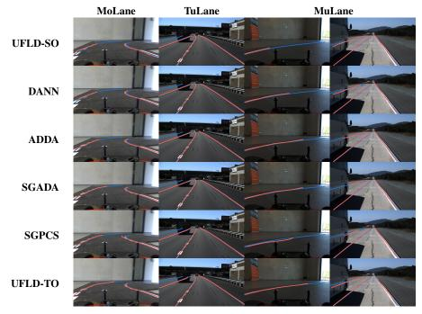
Figure 5: Qualitative results of target domain predictions. Images are randomly sampled. Ground truth lane annotations are marked in blue, predictions in red.
