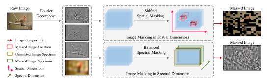
Figure 2: **Overview of the proposed MaskedGAN**: MaskedGAN randomly masks certain image information for effective GAN training with limited training data. We develop two masking strategies that work along orthogonal image dimensions, including *Shifted Spatial Masking* that masks images along spatial dimensions with random shifts and *Balanced Spectra Masking* that masks certain image spectral bands based on self-adaptive probabilities.
