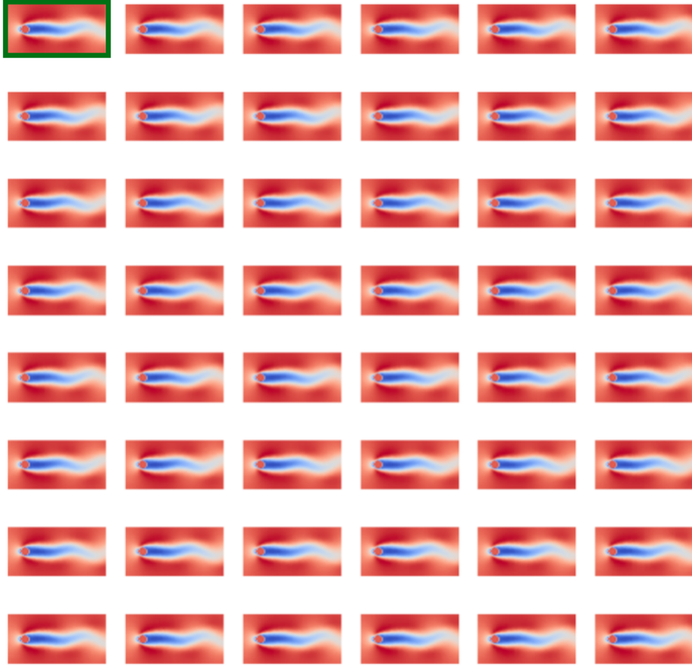
Figure 9: Prediction of the x-momentum. The top-left frame is the last frame of the 16 frame-long sequence that was used to build the dynamics matrix A . All the following frames are predicted.
