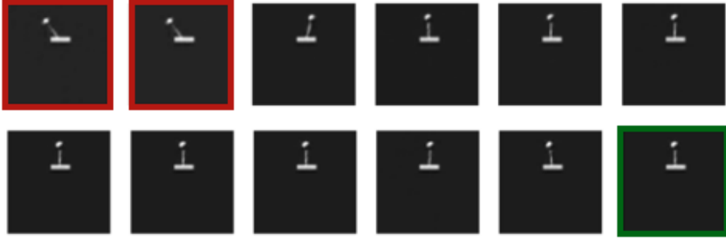
Figure 7: Illustration of cartpole control. Starting from an initial state specified by two consecutive frames (in red), we estimate and apply the controls necessary to guide the pole to an inverted position in a horizon of 0.5 s. The last frame shows the final position of the cartpole after all controls were applied (in green).
