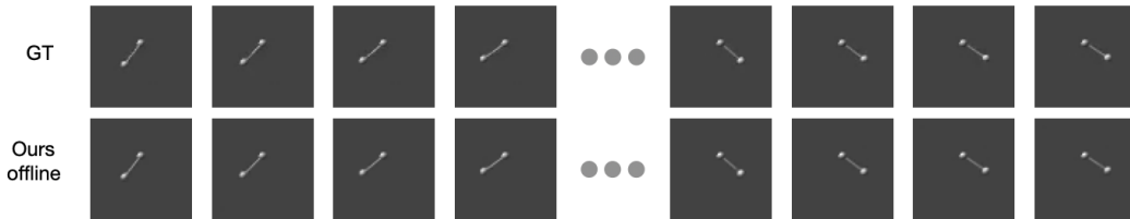
Figure 1: Prediction for the pendulum with low oscillations amplitude (between \frac{\pi}{2} and \frac{3\pi}{2} radians) on a dataset of pendulums of length varying between 0.3 m and 0.8 m. The first row shows ground truth (GT) images. The second row shows predicted frames with our model without updates. In the case of this simple system, our model without updates is enough.
