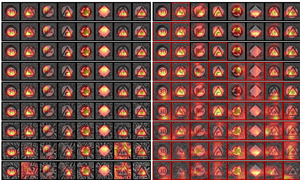
Figure 10: Grad-CAM visualizations for the PGD background perturbation ablation studies (initialized using the bias heuristic). Full (left) and real2sim (right) methods as perturbations increase over \epsilon = 0, 2, 4, 8, 16, 32, 64, 128, 255 (in order from top to bottom). Regions in yellow are more important to the classifier output. Misclassified images are marked with red boxes.
