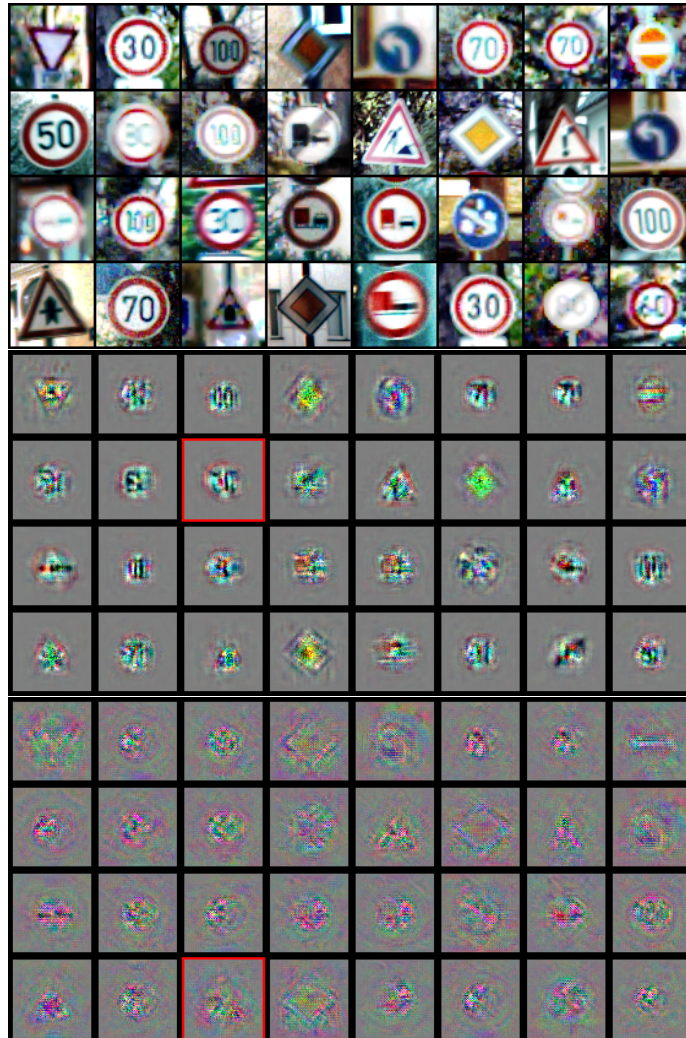
Figure 11: Guided Grad-CAM visualizations for the full (middle) and real2sim (bottom) methods on the GTSRB test set (original images on top). Regions with color visualize the fine-grained features that contribute to the classifier output. Misclassified images are marked with red boxes.
