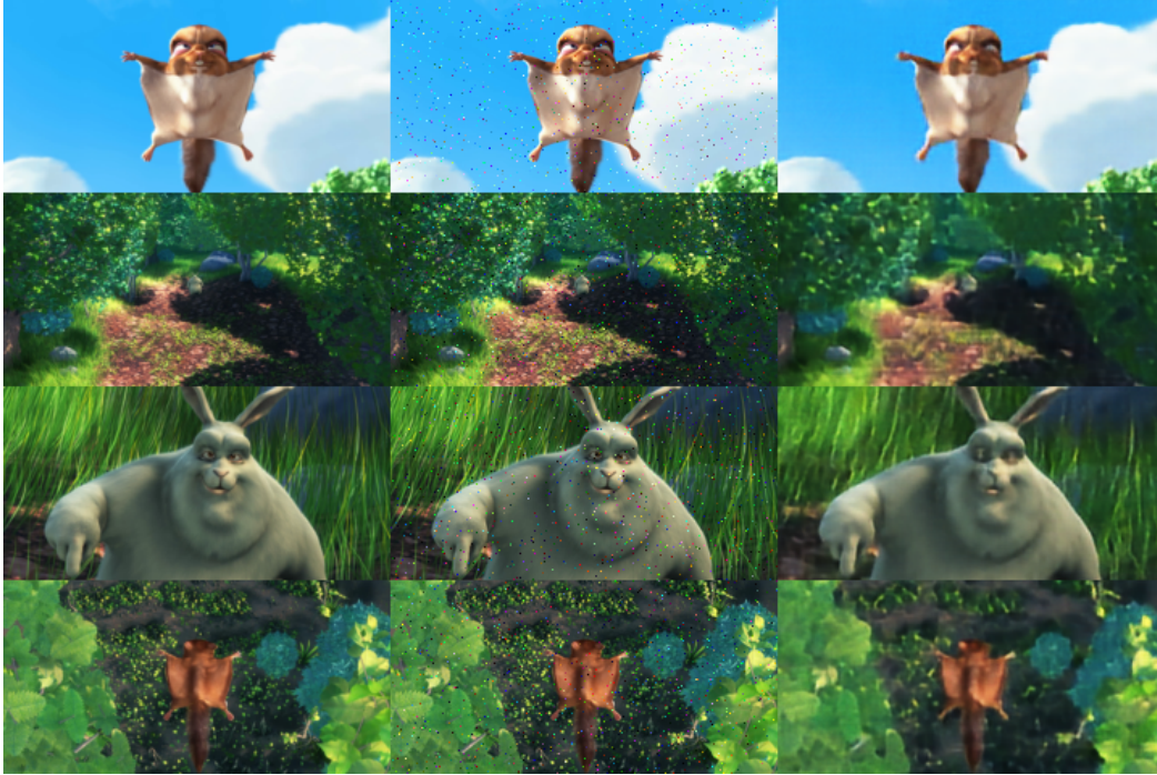
Figure 3: Denoising visualization. Left: Ground truth; Middle: Noisy input Right: NeRV output.
