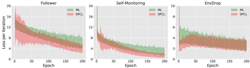
Figure 5: Loss landscape of normal machine learning (ML) and self-paced curriculum learning (SPCL) trained agents. At a particular training epoch, we record the maximum and minimum iteration loss, i.e. an average loss of batch samples. We plot the distances between the two as the shadowed area between lines.
