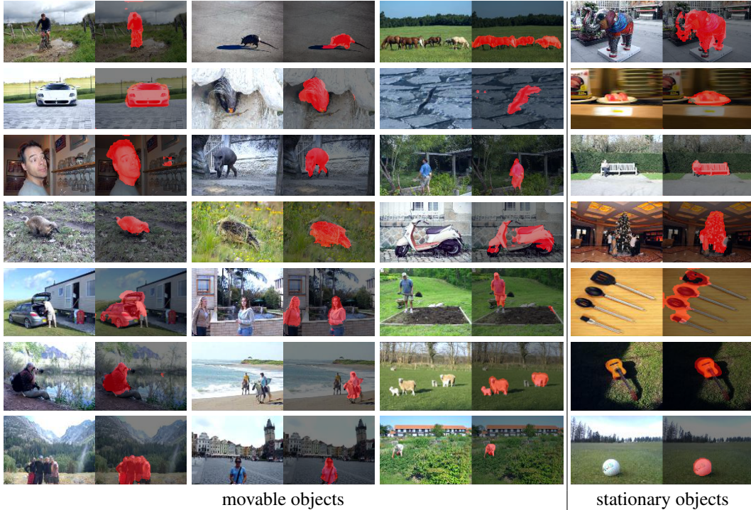
Figure 4: Sample salient object detection results. We directly apply our pretrained segmentation network to novel images in DUTS without any finetuning. Surprisingly, we find that the model pretrained on videos to segment moving objects can generalize to detect stationary unmovable objects in a static image, e.g. the statue, the plate, the bench and the tree in the last column.
