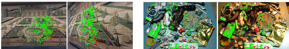
Figure 4: Qualitative results on HPatches. Top 2000 matches are selected with t = 3 pixels. Our method is robust to huge viewpoint (left pair) and illumination (right pair) changes. Green and red dots denote correct and incorrect matches respectively (best viewed in PDF with zoom).
