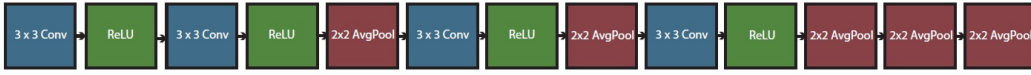
Figure A.7: Details of Myrtle-5 architecture. The network only uses convolutions and average pooling. In particular, we do not use any batch-normalization [5] layers in this network. The figure is borrowed from [11].
