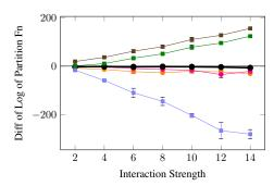
(a)  $4 \times 4$  Ising model with positive interactions. We plot the difference from ground truth (black line at 0). MF-VI approaches ln(1/2) (dotted line) since it only covers one of two symmetric modes for the positive interaction case.
