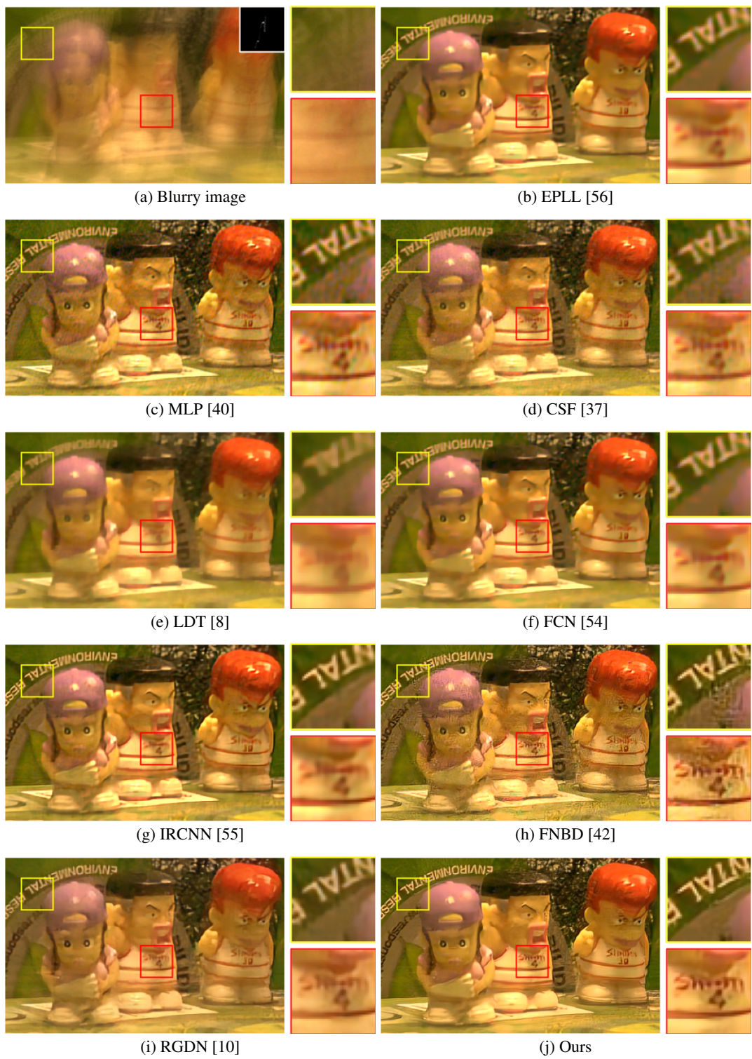
Figure 21: Example with real camera shake from [50]. The blur kernel in (a) is estimated by the method of [29]. The deblurred results by [40, 42] have severe artifacts as shown in the yellow and red boxes of (c)–(h). For other methods, fine-scale structures and detail are over-smoothed. Compared to existing methods, our method recovers much clearer characters as shown in (j).
