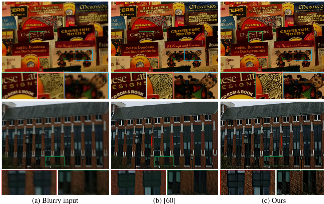
Figure 9: Examples with non-uniform image deblurring. The images shown in (b) are obtained from the reported results of [60]. Compared to the results in (b), the images recovered by our method in (c) are much clearer with finer detail.
