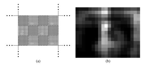
Figure 6: (a) Stage 2 network for computing local changes in contrast. Blocks of  $8 \times 8$  IFAT neurons from stage 1 (shown as regions alternately shaded white and gray) project to single IFAT neurons in stage 2 (not shown). Blocks are shown as non-overlapping for clarity. (b) Output of stage 2, as implemented on the IFAT, with Figure 5b from stage 1 as input.
