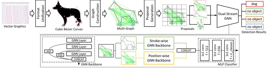
Figure 2: The overall pipeline of the proposed method.
