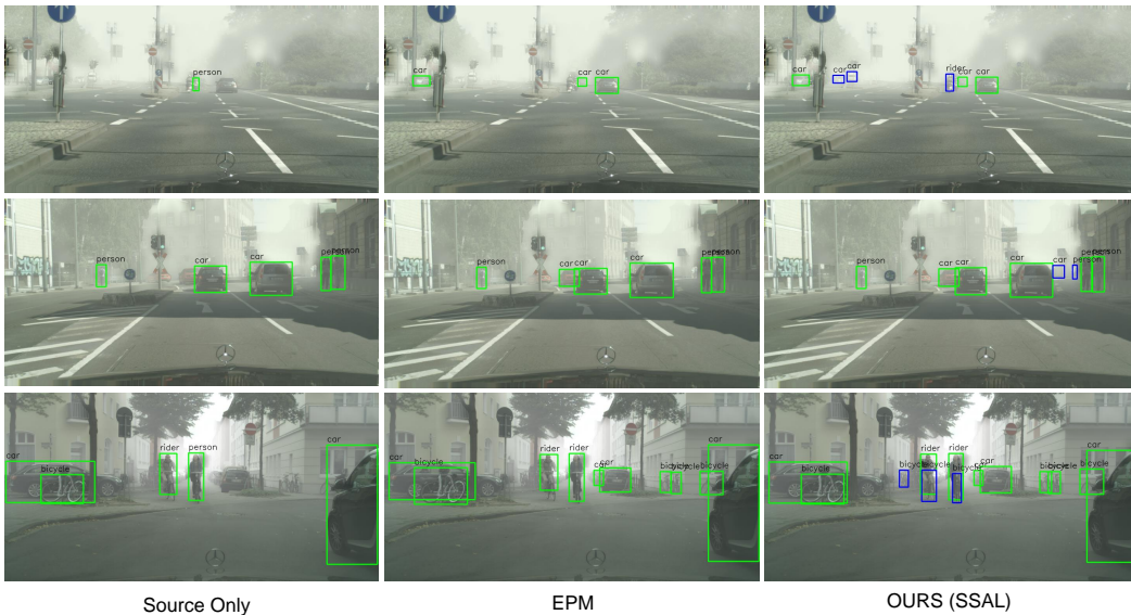
Figure 5: Detections missed by the EPM and found by our method are shown in Blue. Compared to EPM [17] our method achieves better adaptation.
