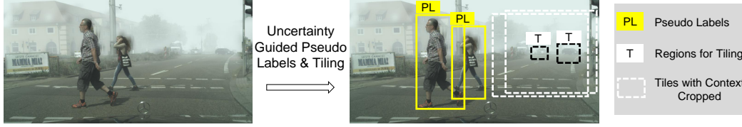
Figure 2: An illustration on which detections will be considered as pseudo-labels and which for extracting tiles. More certain detections, such as pedestrians are taken as pseudo-labels, whereas relatively uncertain ones, like cars under fog, are used for extracting tiles.
