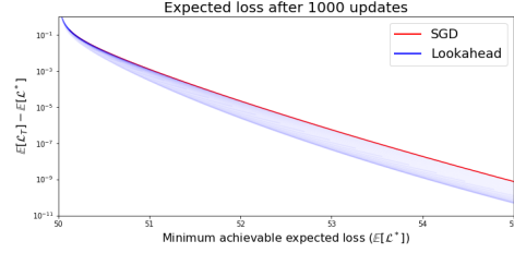
Figure 3: Comparing expected optimization progress between SGD and Lookahead( k = 5 ) on the noisy quadratic model. Each vertical slice compares the convergence of optimizers with the same final loss values. For Lookahead, convergence rates for 100 evenly spaced \alpha values in the range (0, 1] are overlaid.
