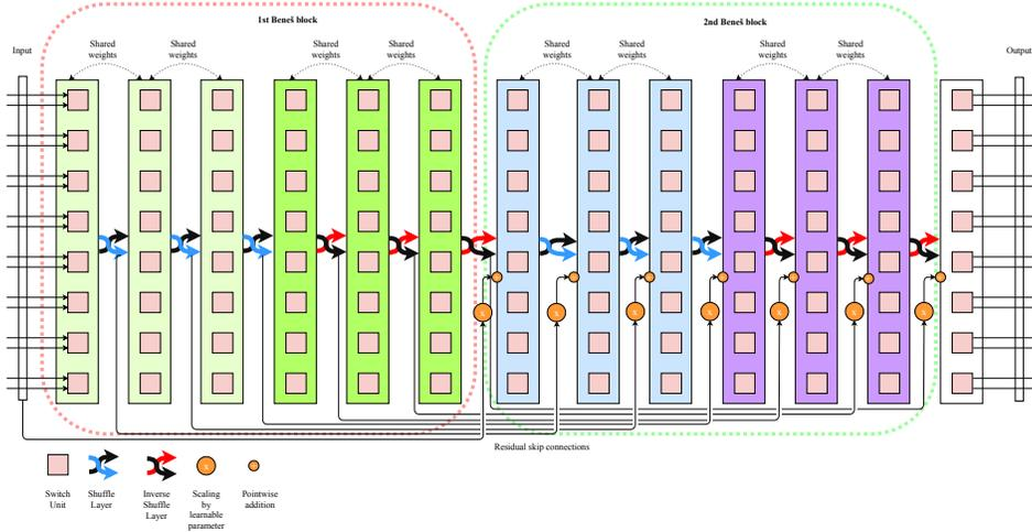
Figure 3: Neural Shuffle-Exchange network with 2 Beneš blocks.
