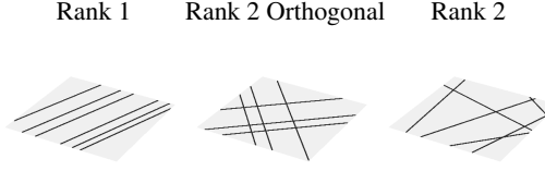
Figure 5: Examples of various weight constraints and their impact on the layer input space partitioning. (Left) A low-rank weight matrix leads to colinear cuts, with the cut spacing determined by the bias values. (Middle) An orthogonal weight matrix leads to orthogonal cuts. (Right) An arbitrary weight matrix leads to an unconstrained partition.
