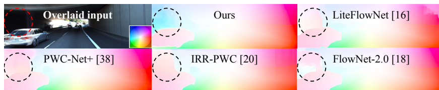
Figure 2: Results on KITTI-15 test image 48. Color indicates the direction and magnitude of the displacements following Middlebury color wheel, as shown in the top-left image. While prior methods predict the dark wall (circled) as moving to the right together with the front vehicle, our method correctly predicts it as moving to the left.
