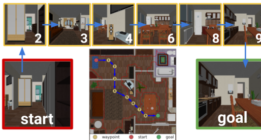
Figure 5: Visual Navigation: Given an initial state and goal state, our method automatically finds a sequence of intermediate waypoints. The agent then follows those waypoints to reach the goal.
