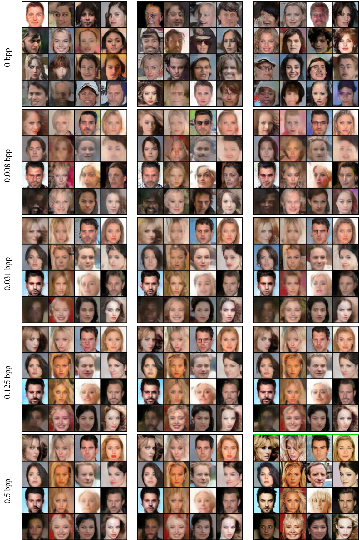
Figure 6: Testing reconstructions produced by our DPLC model with WGAN-GP G^* , along with the original image (green border), for CelebA. The variability between different reconstructions increases as the bitrate decreases.
