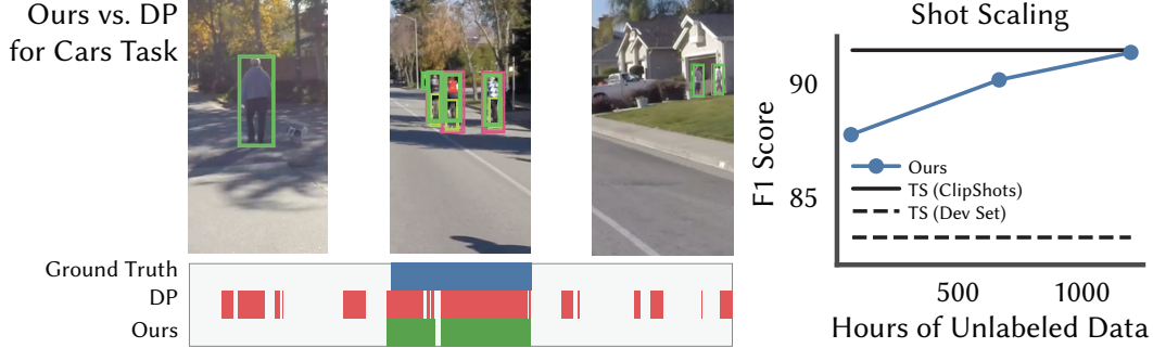
Figure 3: (Left) Dugong has fewer false positives than data programming on a cyclist detection task since it uses sequential correlations and distributional knowledge to assign better training labels. (Right) Increasing unlabeled data can help match a benchmark model trained with 686\times more ground truth data, i.e., using traditional supervision (TS).
