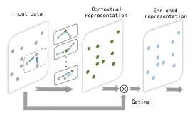
Figure 2: The point enrichment process relies on our proposed gated fusion strategy to enrich the point representation by considering the neighbouring and contextual points of each point.
