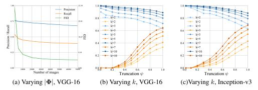
Figure 3: (a) Our metric behaves similarly to FID in terms of varying sample count. (b) Precision (blue) and recall (orange) for several neighborhood sizes k. Larger k increases both numbers. Here a trained model ( $\psi=1$ ) was expanded to a family of models by artificially limiting the variation in the results. We would expect the precision and recall to reach 1.0 and 0.0, respectively, when  $\psi\to0$ . (c) Using Inception-v3 features instead of VGG-16 yields a substantially similar result.
