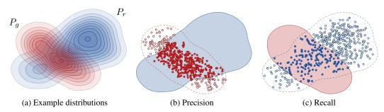
Figure 1: Definition of precision and recall for distributions [24]. (a) Denote the distribution of real images with  $P_r$  (blue) and the distribution of generated images with  $P_g$  (red). (b) Precision is the probability that a random image from  $P_g$  falls within the support of  $P_r$ . (c) Recall is the probability that a random image from  $P_r$  falls within the support of  $P_g$ .
