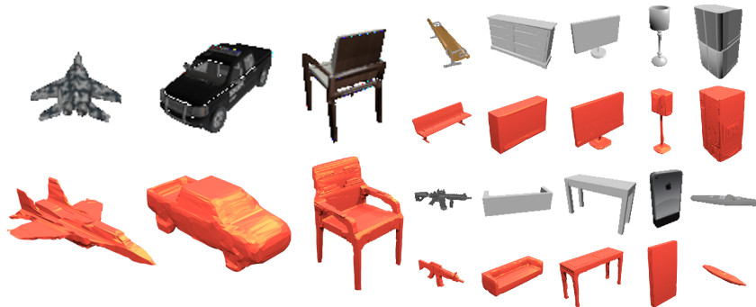
Figure 6: 3D object reconstruction 256^3 rendering results from our method, MVD (bottom), of the 13 classes from ShapeNet, by interpreting 2D image input (top).
